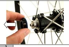
Remove the adjusting sleeve, to be subsequently refitted.
