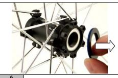
Remove the protective cover of the axle disk side.
