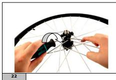
Proceed to tightening the allen screw with a torque screwdriver calibrated to 2.5 Nm (22 in.lbs). To reach the pre-set torque, wait for the wrench to click.
