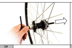
Insert the threaded axle inside the hub body of the wheel, bringing the axle out from the opposite side.
