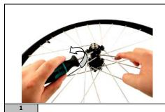
Use a 2.5 mm allen wrench to loosen the screw of the hub adjusting sleeve.
