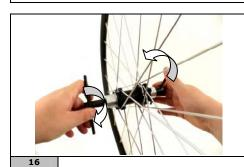
Tighten the tool until the bearings are fully pressed into the hub seats.
