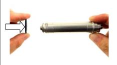
Insert the non-drive side protective cover on the hub axle. The flat part faces the outside of the hub.
