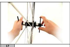
Loosen the guide for pressing the bearings and remove the threaded axle from inside the hub body.
