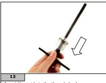
Insert the guide in the threaded axle.
