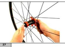
Insert two hex wrenches inside the hexagons of the hub body and tighten with force. Hold the wrench on the right (side opposite the adjusting sleeve) still; turn the one on the left clockwise.
