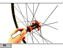
Tighten the fixing bolt on the hub axle. Be sure to
